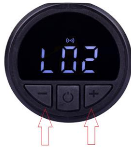
"+", "-" buttons, switch PAS level
