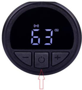
power button, power indication by default
